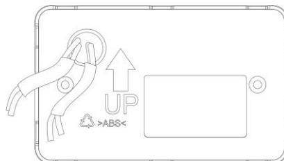
Cover the wires coming from mains using the sheaths provided inside the box.
