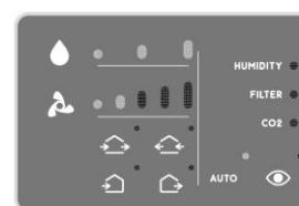
It is possible to change the threshold level of the humidistat, pushing "H" button, to adapt the value to the type of the environment in which is installed. Once the humidity value set is overtaken, the product continuously extracts air at the maximum speed until the humidity level returns below the pre-set value. In case of more units, all the products will automatically run extraction until the restoration of the threshold value.
