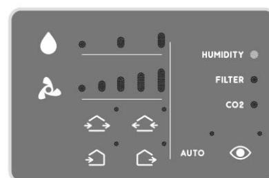
**AC – ALARM: Exceeded CO<sub>2</sub> threshold set**
