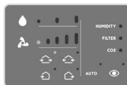
V1 – V2 – V3      Steady light based on the set speed
