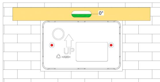
Fix the device on the wall with two screws.
